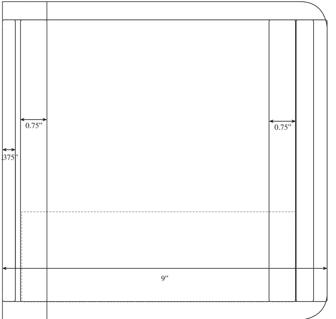
The standard clearance from the front of the control panel is  $\frac{7}{8}$  inch.  $\frac{1}{2}$  is filled up by the front panel and the rest is to keep the control knobs, switches and logo from being hit, bent, broken, etc...
