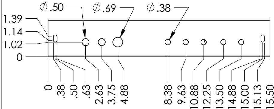
ONE 5G15 ENDCAP TO BE SPOT WELDED IN EACH END OF CHASSIS.
