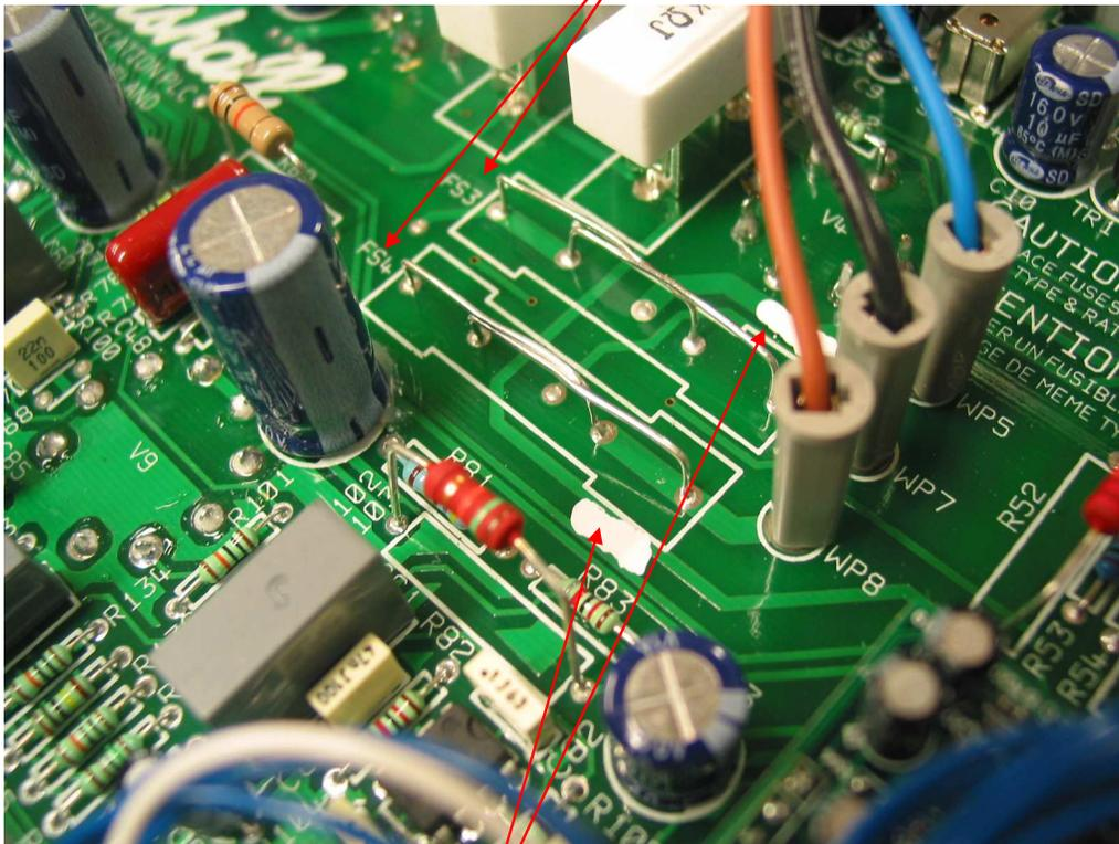
2. Cover fuse ratings of FS3 & FS4 (T10A) marked on PCB silk screen with TIPP-EX.
