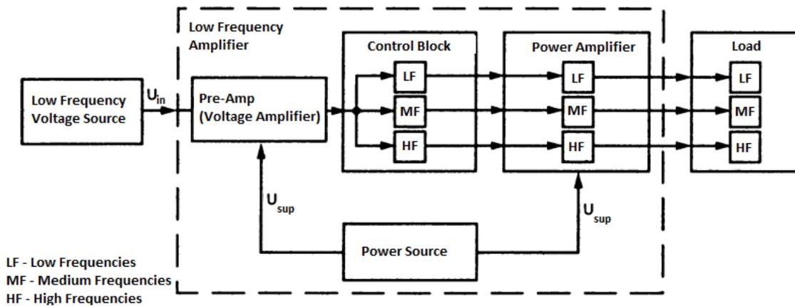
Figure 9. The structure of multistage low-frequency amplifier with control block which separates signal on different frequency channels. [12]
