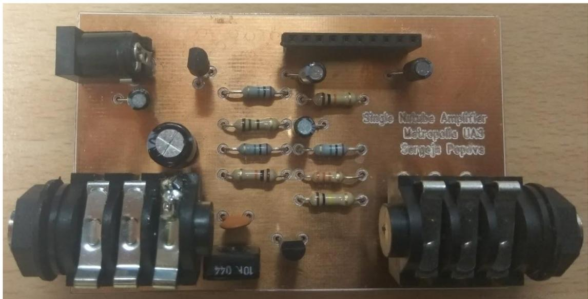
Figure 14. Single stage, single channel Nutube amplifier.
