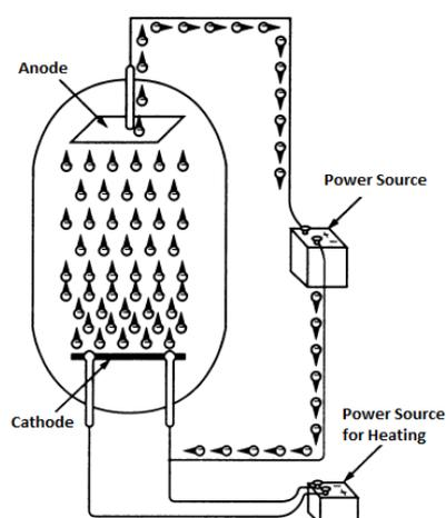
Figure 6. Electron movement inside vacuum tube [12]
