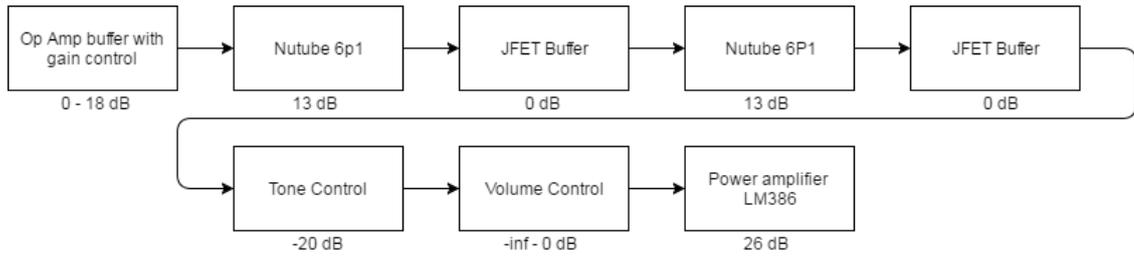
Figure 22. Block diagram of portable Nutube amplifier with valve distortion
