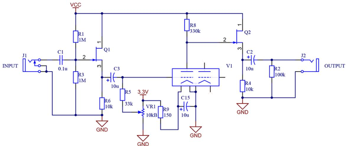
Figure 13. Schematic of single Nutube 6P1 amplifier by Korg.
