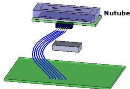
Figure 4. Preventing microphonic noises from the main board. [15]
