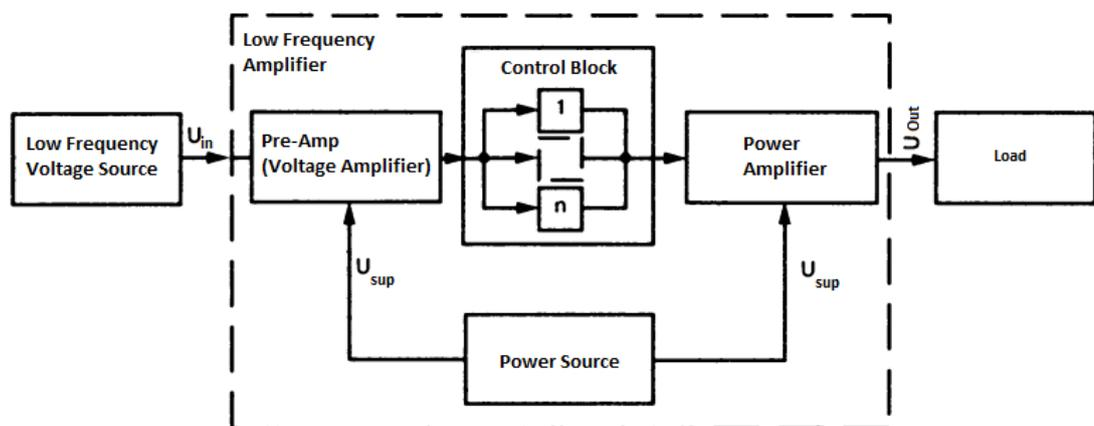
Figure 8. The structure of multistage low-frequency amplifier with control block. [12]
