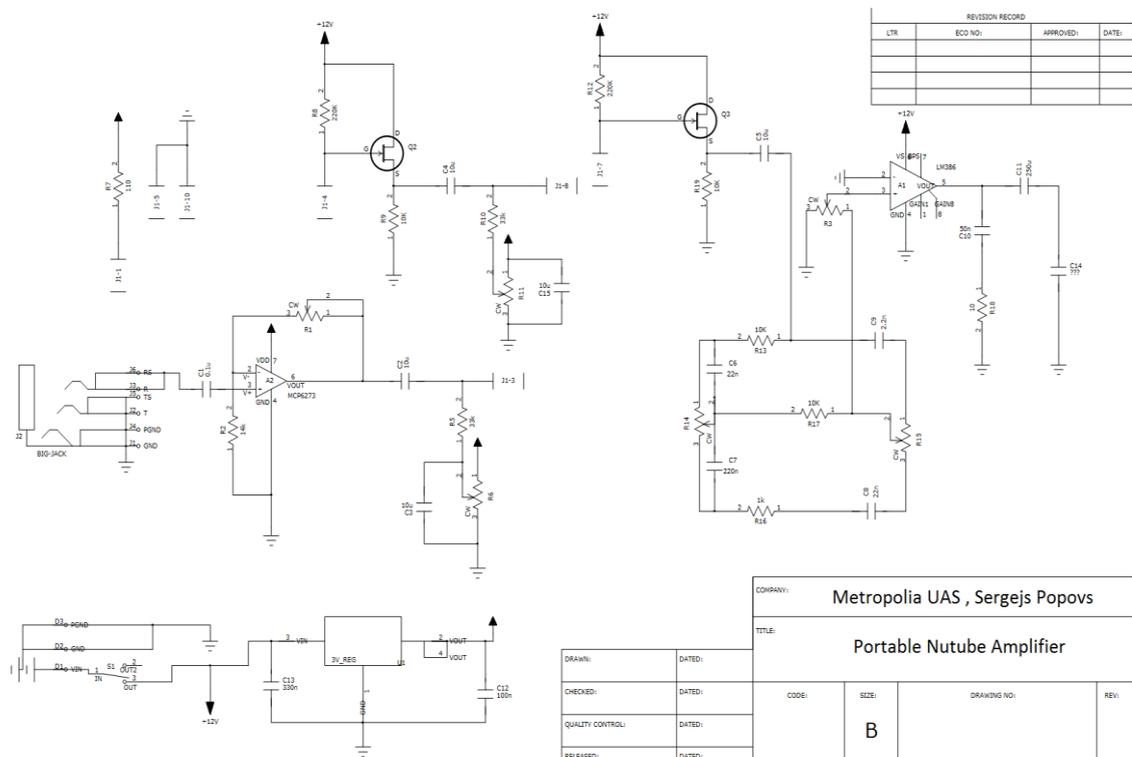
Figure 23. Schematic of Portable Nutube Amplifier
