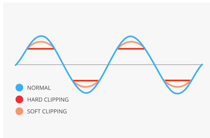
Figure 16. Sine wave under hard clipping and soft clipping distortion.
