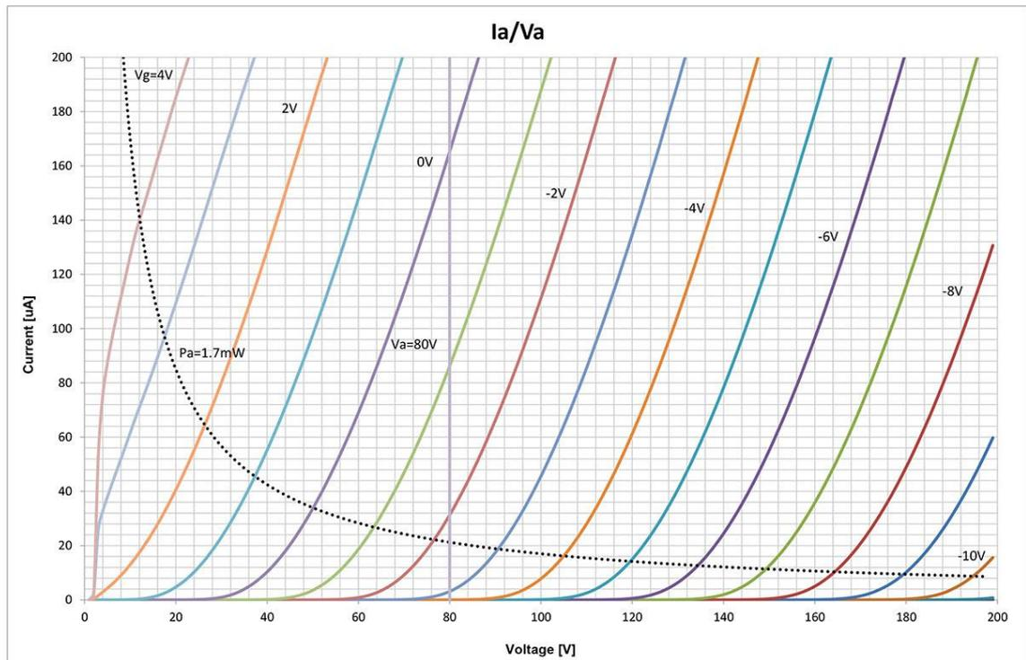
Figure 2. Anode characteristics of Nutube. Dependence of anode current on anode voltage [14]
