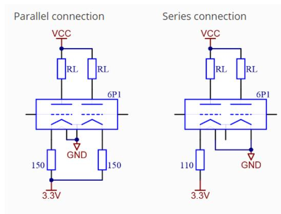
Figure 3. Filament connection in parallel and in series. [15]
