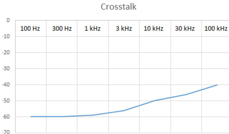
Figure 25. Graph of crosstalk attenuation on Nutube 6p1 stereo 12W Nutube amplifier. Measured crosstalk attenuation is around 56 dB in Nutube Stereo 12W amplifier. HiFi minimum requirement is >30 dB for 250 Hz and >40 dB for 10 kHz. In this case, stereo amplifier passes minimum requirements. With frequency increasing this ratio is increasing, because output voltage amplitude decreases as well and this amplifier works as low pass filter because it's audible effective frequency range.
