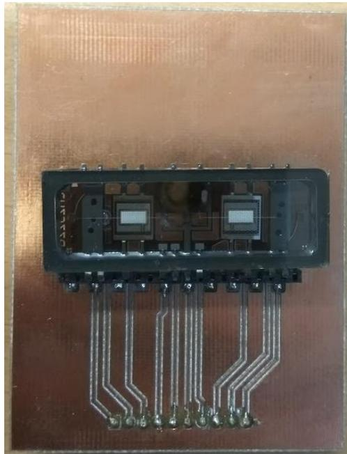
Figure 10. Nutube mounting board.
