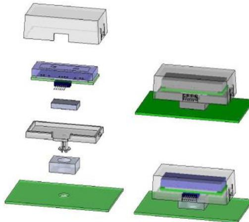
Figure 5. Preventing microphonic noises from the air(sound). [15]
