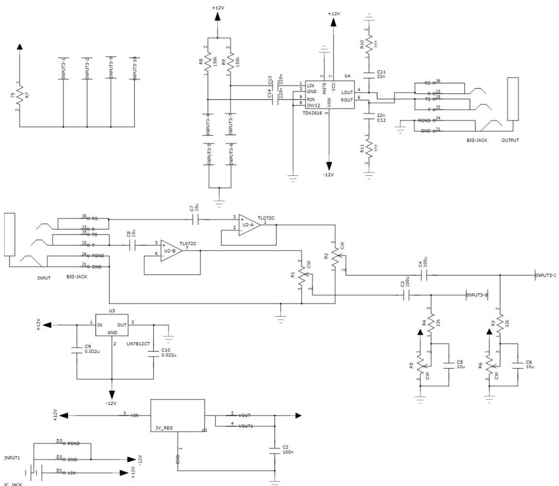
Figure 19. Stereo 12W amplifier with Nutube preamp.
