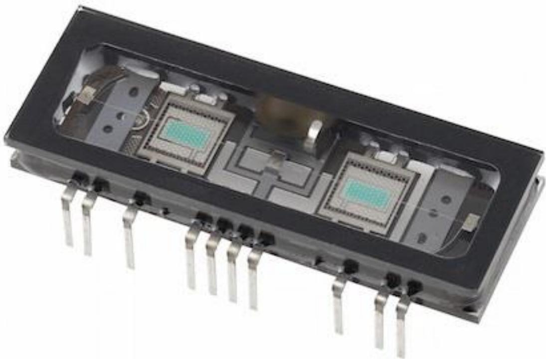
Figure 1. Nutube 6P1 produced by Noritake for Korg. [15]
