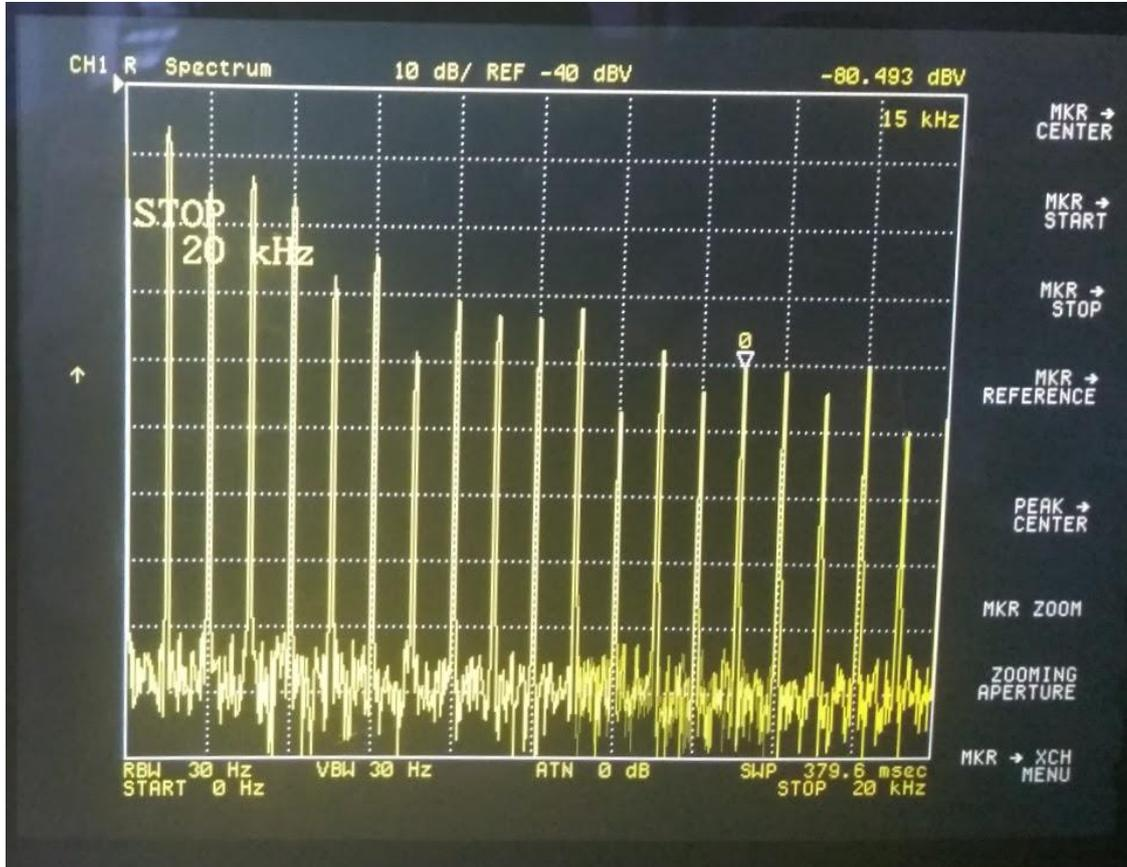
Figure 24. The output of the spectrum analyzer with input signal frequency of 1 kHz.
