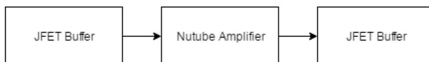
Figure 12. Block Scheme of Single Stage Nutube Amplifier by Korg
