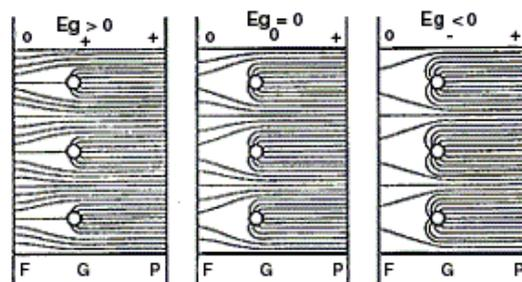
Figure 7. Change of current flow through the grid, depending on voltage on the grid [12]
