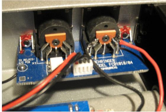
It is VERY IMPORTANT that the red wire have positive voltage supplied to it and the black wire have negative voltage supplied to it. The phantom adapter has a voltage regulator on it that needs to have positive voltage on the red wire. If you are also buying the optional insertion cable the red and black wires must be hooked up as stated above because the insertion cable is wired in respect to the positive voltage (red) being on the right and negative voltage (black) being on the left.
