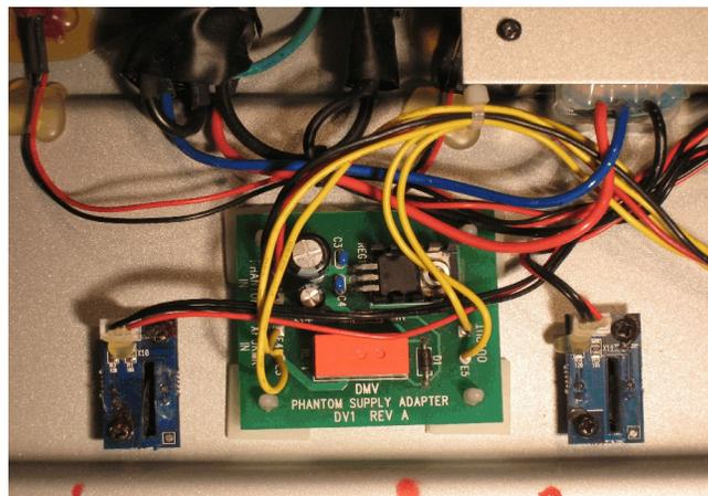
8. Route the two yellow wires that came pre-attached to the phantom supply adapter back to the location where you un-soldered, or cut, the yellow wires that were attached to the FCB1010's printed board. Once again, make sure to route the wires so that they will not interfere with the operation of the expression pedal's optical strips.
