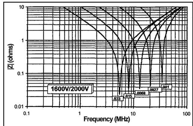
Please note: Capacitance values above are in  $\mu\text{F}$ . The resonant frequency and impedance shown above apply to units with a 0.250" lead length and are typical values only. Please contact us for data on the 100VDC rated units.
